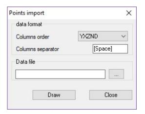
In this window User may select format of file with data, columns order and separator of columns, also User may select file with data. After click button [Draw], application will insert points, numbers and blocks symbols if contained on data file.
