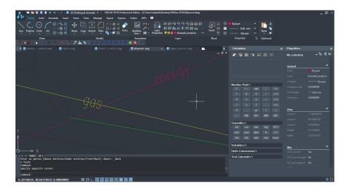
This command help You to make drawing more readable by covering objects under MText by wipeout. All You need to do is run command and select MText entity. Everything under this MText will not be visible, but it will there like line on picture above, will not be split into two separate lines but only not visible in rande under MText.
